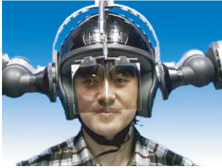
Fig. 12. General view of a head mounted projector.
