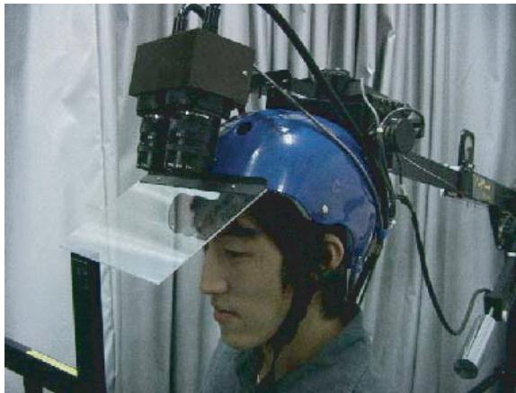
Fig. 22. General view of head-mounted projector used in this configuration.
