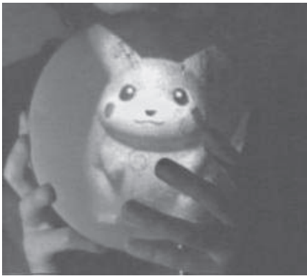
Fig. 13. Projected image on a spherical retro-reflective screen.
