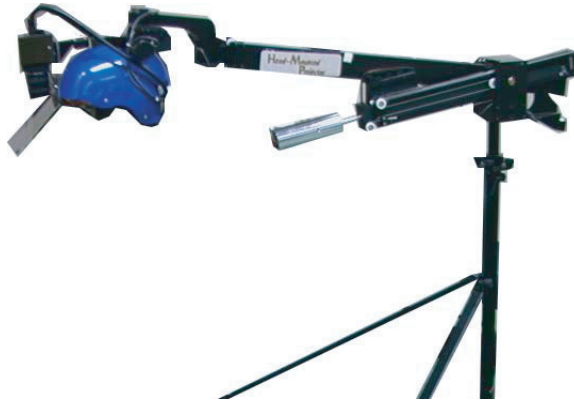
Fig. 21. General view of head-mounted projector suspended by counter-balanced goniometer with 6-DOF.
