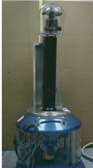
Fig. 19. General view of stereo camera mounted on torso mechanism with 6-DOF.
